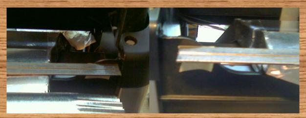
I marked the lines on the top side of the ruler. This will give the needed clearance so that the clear cover does not rest on the insert. Also mark the cover at each side of the insert. I used masking tape to mark the lines as it is easier to see the mark line with the tape on the black surface.
