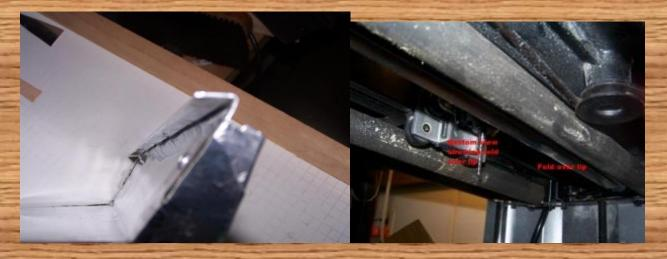
Install and tighten the TWO 4 MM screws to hold the insert in place.
